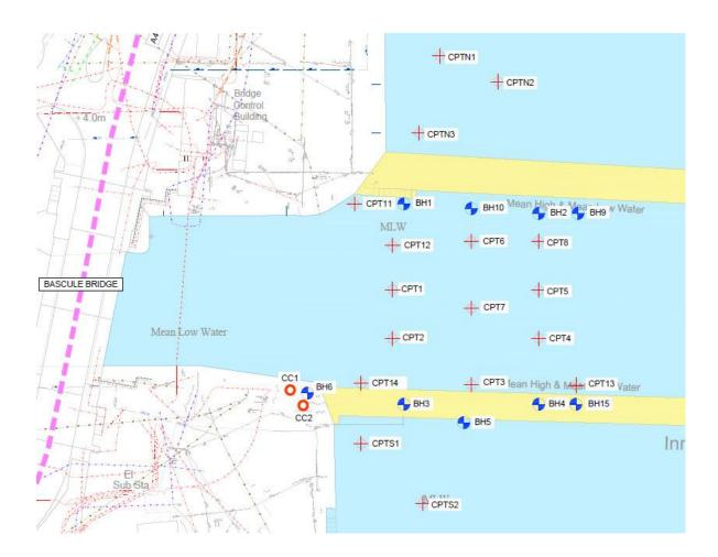
The GI works are now scheduled to take until approx. 6<sup>th</sup> March, but may further over run subject to weather and operational delays. Works will involve jack up barge Sandpiper being positioned in the various locations, to undertake the Cone Penetration Tests (CPT), and Boreholes (BH). Works will be undertaken 24/7.
