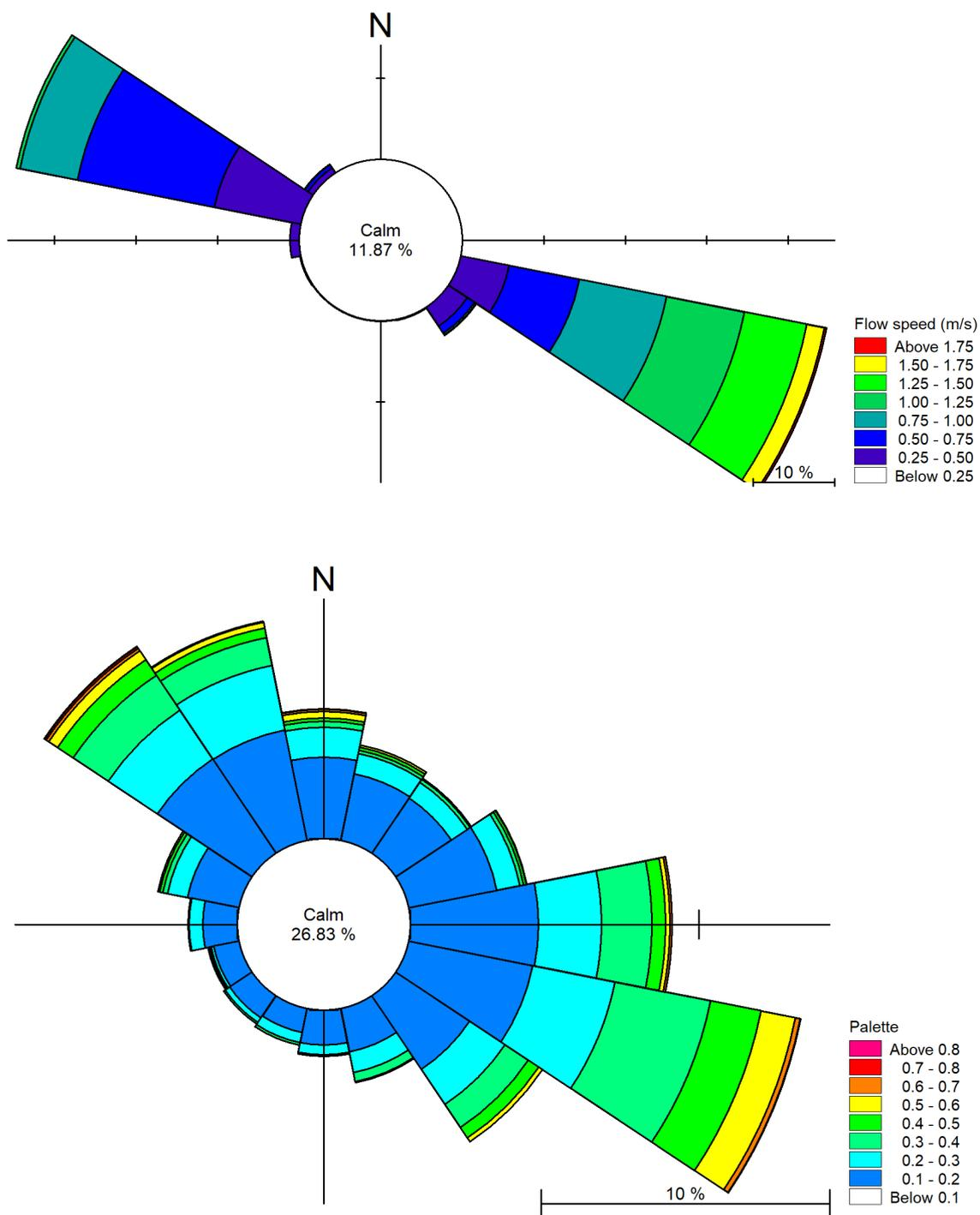
**Figure 6. Current rose (top) and wave rose (bottom), based on measured data collected between November 2019 and June 2020**
