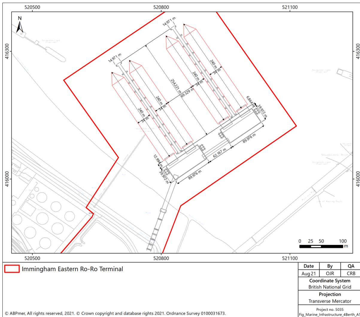
**Figure 2. Layout of proposed marine works at Immingham Eastern Ro-Ro Terminal**
