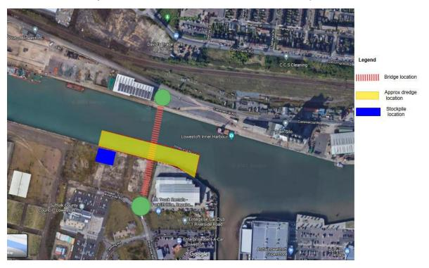
Dredging will be undertaken via a long reach excavator working from a 20m x 12m spud leg barge 'NEVA', transferring spoil to 2 x small 16m x 3.5m hopper barges.
