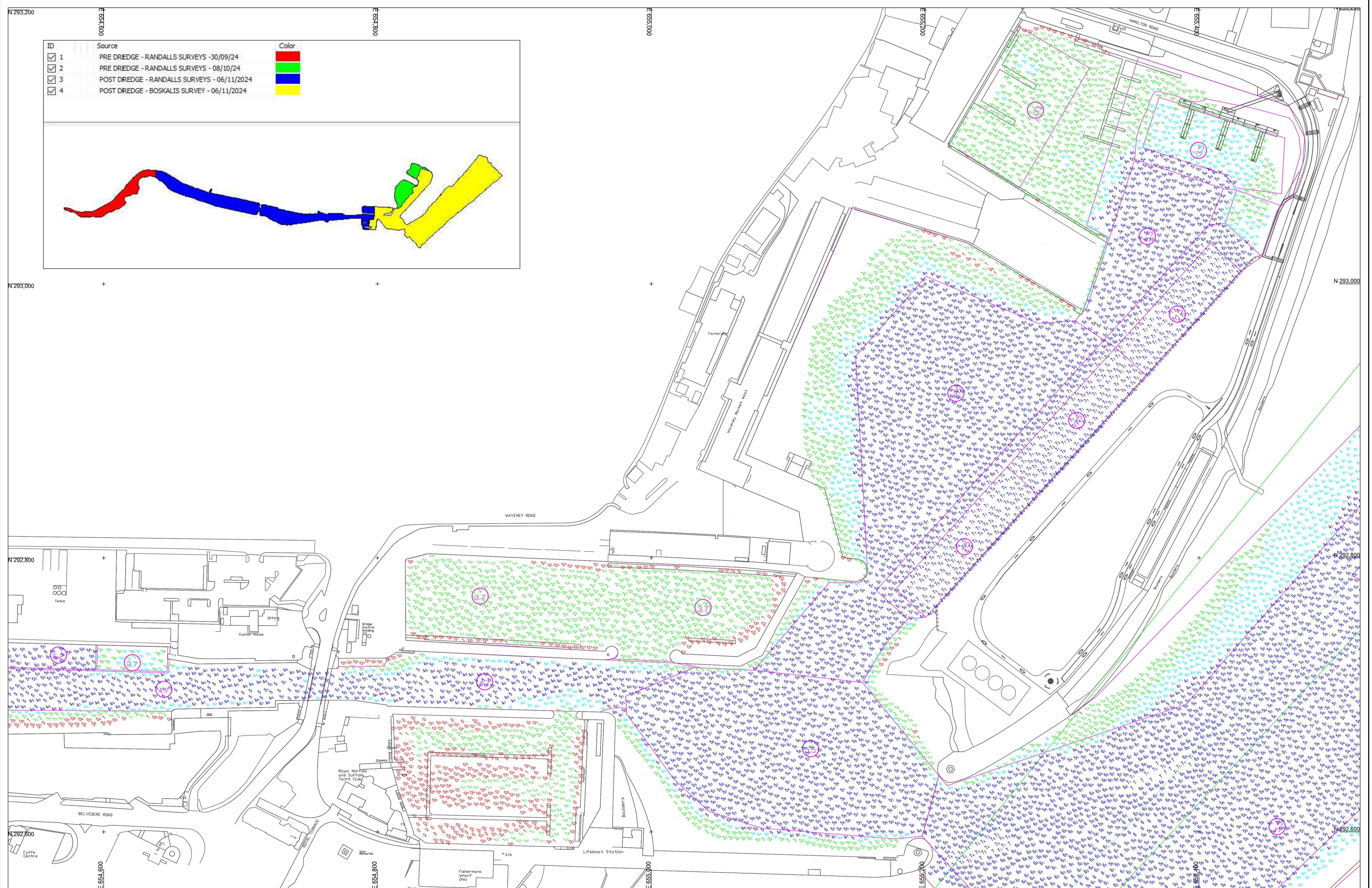
**DATUM FOR SOUNDINGS:** Soundings are relative to Admiralty Chart Datum (A.C.D.) A.C.D is 1.5 metres below O.D. Newly Negative numbers indicate heights above datum. Positive numbers indicate depths below datum
