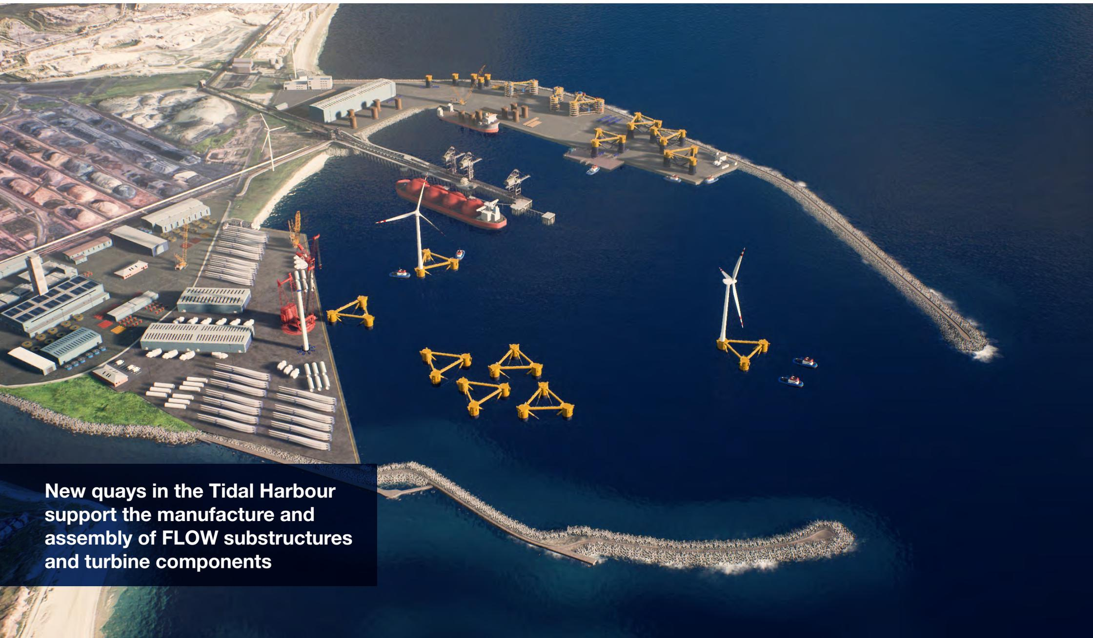
**New quays in the Tidal Harbour support the manufacture and assembly of FLOW substructures and turbine components**
