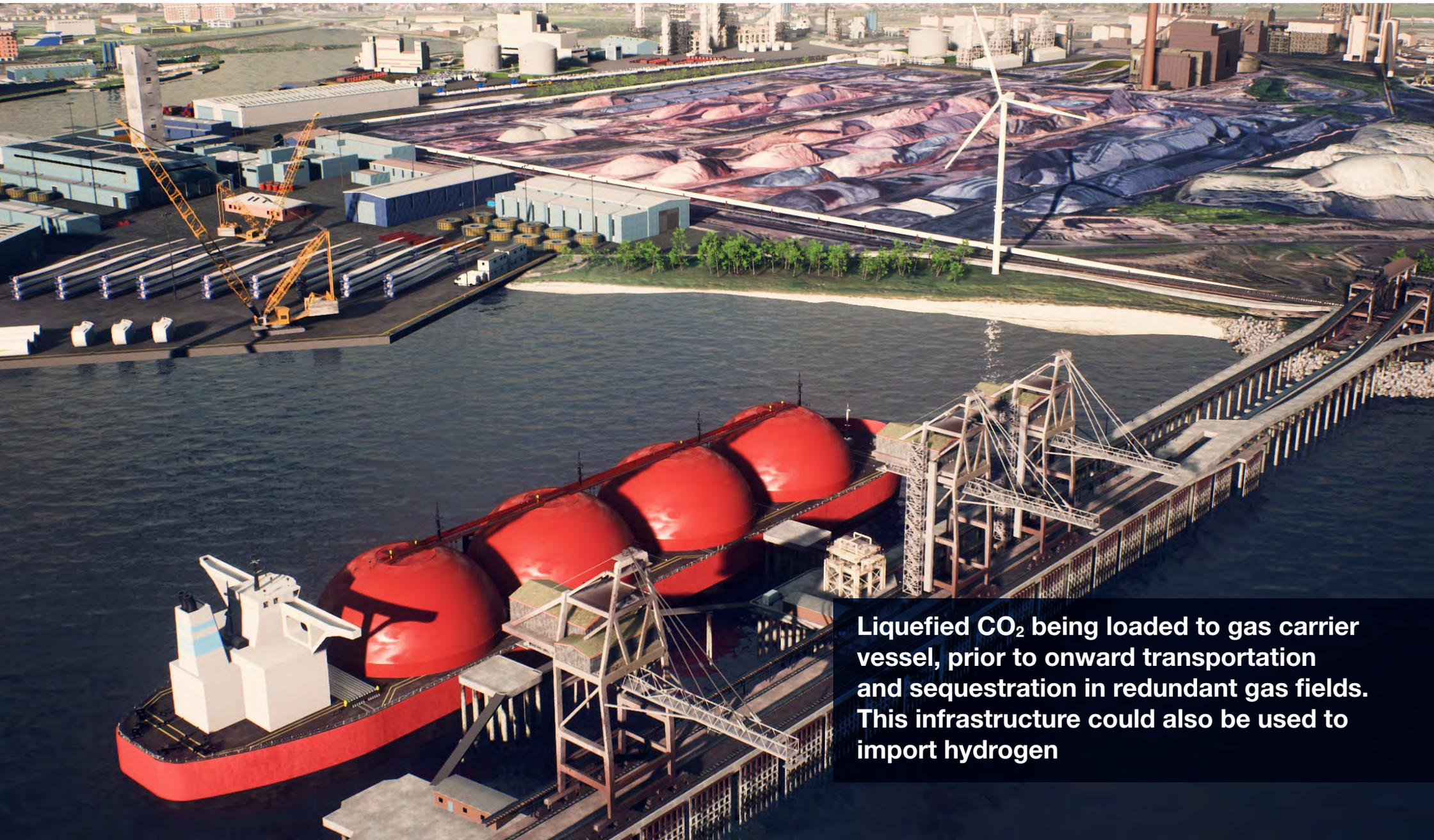
Liquefied CO<sub>2</sub> being loaded to gas carrier vessel, prior to onward transportation and sequestration in redundant gas fields. This infrastructure could also be used to import hydrogen
